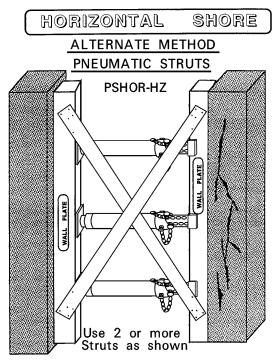
See previous sheet in this Section-Wood Horizontal Shore for Wall Plates. and Diagonal Bracing See Strut Tables, Sect 7, Struct. Spec FOG for Recommended Strut Loading, based on Height (Length) HAND TIGHTEN HORIZONTAL STRUTS EXCEPT WHEN USED AS TRENCH SHORES
