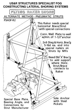
See previous pages in this Sect.for Notes on Wood Flying Rakers. These Rakers are weaker than Full-Ht Rakers, but may be useful as Initial, Spot Rakers
