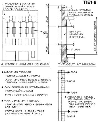
\* TIEBACKS COULD BE EXTENDED ACROSS BLOG TO OPP WALL AND ANCHORED. OR ANCHORED TO FLOOR BEAMS.
