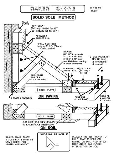
Design Load for 1- Pair of Raker Shores w/ Bracing is 5,000 lb
