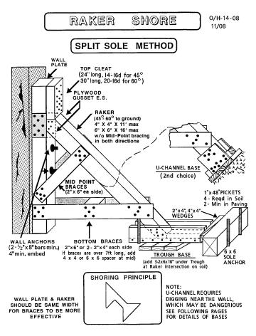
Design Load for 1- Pair of Raker Shores w/ Bracing is 5,000 lb (Trough Base is Preferred, since No Digging is Required next to Dangerous Wall. Add 18" sq. Wood Foot under intersection of Raker & Sole if bearing on Soil)
