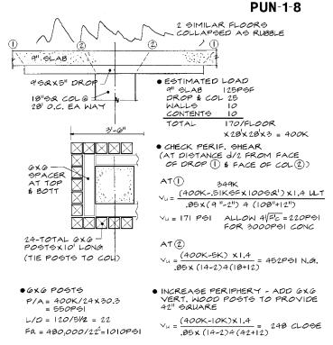
POSTS FIGURE FOR PERP. TO GRAIN BEARING (730PG) MAX) SO SHIMS & SPREADER MAY BE USED. LOAD MUST BE SPREAD TO FLOORS BELOW (THRU PERIF SHEAR OR ON TO EXISTING FOOTING. ONE MUST ALSO CONSIDER IF THE SLAB SHOULD BE SHORED AT MID-SPAN ETC. BY OBSERVING CRACKS SINCE THEY ARE NORMALLY VISIBLE FROM BOTTOM OF SLAB.
