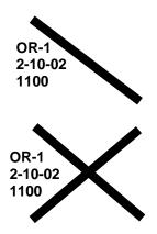
Single slash drawn upon entry to a structure or area indicates search operations are currently in progress. Upon entering a building or a separate wing of a large building, add the Search Team I.D., Date and Time (24hr) of entry. (Next to main entry)
