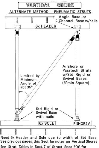
Recommended Strut Loading, based on Height (Length) MAX AIR PRESSURE = 50 PSI, SEE WARNING Pg 3-32 HAND TIGHTEN ALL PNEUMATIC STRUTS - SNUG TIGHT
