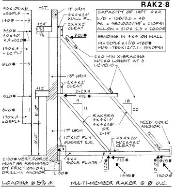
WALL LEANING ABOUT 16" AT TOP OF 27' HEIGHT WOLLD BE5% OUT OF PLUMB. ITS UNREALISTIC TO THINK ONE WOLLD FIND A URM WALL THAT 16 MORE OUT OF PLUMB AND HAS NOT COLLAPSED. DUE TO POSSIBLE ADDITIONAL LOAD FROM AFTERSHOCK IT 16 RECOMMENDED THAT THE SHORES & CONNS. FIGURE FOR 10% (FORCES SHOWN WOLLD DOUBLE)
