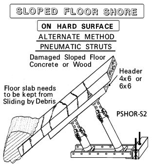
Struts by Airshore or Paratech with Angle Base or Channel Base to Header Sole is Raker Wall Channel with Std Raker Connections and Bearing Angle against Sole Anchor
