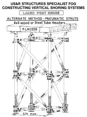
This configuration of Struts is intended for use where wood Laced Post Sys are not available. The Horiz. & Diagonal members must be able to resist, both Tension & Compression Forces.
