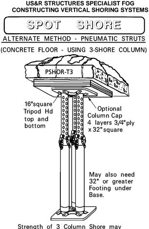
Strength of 3 Column Shore may be taken as 3 times the values given for individual Struts of same height in Sect.7 of Struct.Spec FOG MAX AIR PRESSURE = 50 PSI, HAND TIGHTEN ALL STRUTS - SNUG
