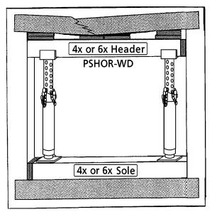
Use min. of 2 Airshore or Paratech Struts Wedges at one end of Header and Sole See previous pages in this Section, Wood Window and Door Shores for Notes, etc. See Strut Tables in Sect.7 of Struct. Spec FOG for Recommended Strut Loading, based on Height (Length)
