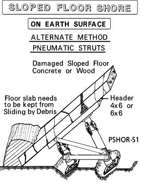
Struts by Airshore or Paratech with Std Swivel Bases or 12"sq Base Plates depending on Soil Strength
