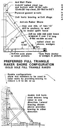
All systems using 4x4 members over 11ft long should be braced in two directions in order to limit L/D to 25±
